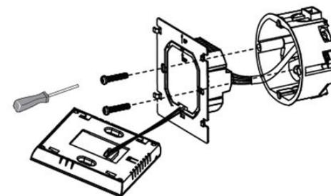
3. Connect the LCD board into the wall plate.
